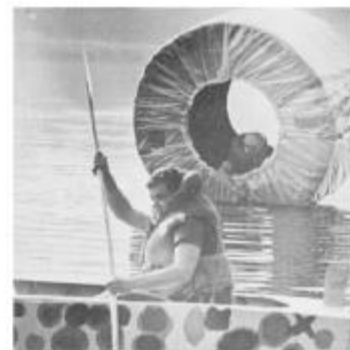
The uniqueness of this design was the use of cardboard to construct the device. In the background a "Hamster Cage" design allows students to run inside as a means of propulsion.
